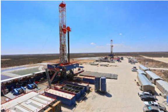
*Figure Caption: New technology has revolutionized drilling, like Patterson-UTI's APEX WALKING® drill rig. This rig uses hydraulic feet to 'walk' from one drill site to another and operates in West Texas.*
