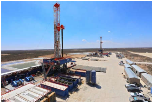
A Patterson-UTI APEX WALKING drilling rig, operating in the Permian Basin, uses hydraulic feet to walk from one drill site to another, able to move forward, sideways or in a circle with pipe racked back, without the need to move other primary equipment. These new technologies have not only reduced cost and increased efficiency, but have played an important role in the evolution of the industry in response to external forces like the recent Saudi-U.S. oil war.
